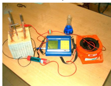
Figure 10 - Appearance of a concrete specimen with installed reinforcement
