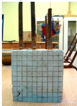
Figure 10 - Appearance of a concrete specimen with installed reinforcement
